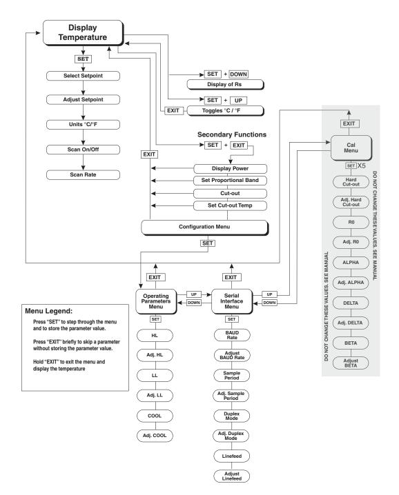
Figure 4 Controller Operation Flowchart
